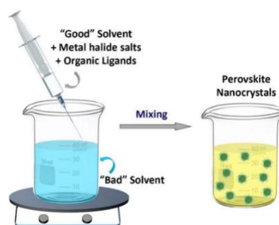
Figure 1.22. Schematic representation of LARP method.
